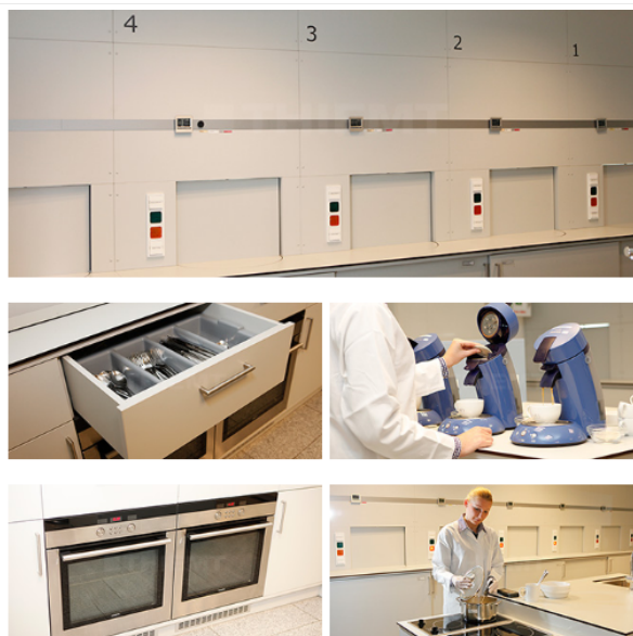
Figure 3 - The backside of the test cabin acts as a wall unit of the preparation room. The samples preparation and coding, such as the presentation takes place right here. The materials of the ceilings, walls, and floors should be odourless and olfactory inert, such as the furnishings.
