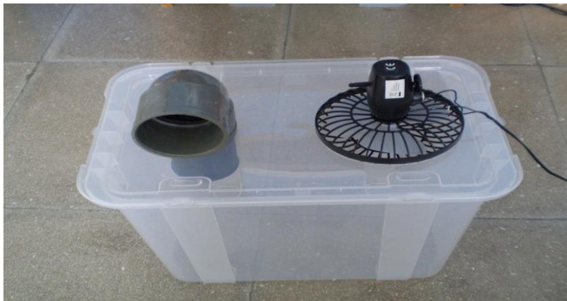
Figure 10. A small car fan and a plastic box repurposed into an ice-based cooler Image used with permission
